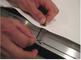
4. Pull and stretch the other side over a post. We have a short video clip showing this procedure on the fixed frame screens page.
