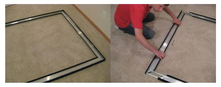
For this fourth piece, a short side, insert its L-brackets but do not tighten at this time. Align the four L-brackets into their mating slots into the top and bottom frame pieces and slide into position.
