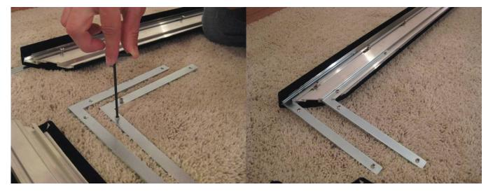
Align the L-brackets into their mating slots in the other frame member, and slide them together making a nice tight corner.
