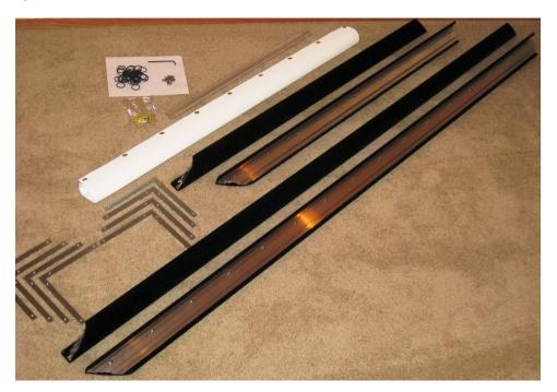
Lay the frame members faced down where they will be installed, together with the corner L-brackets. Put the set screws and the hex key on a piece of paper or dish so you don't lose them.
