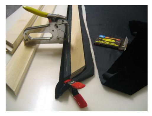
After you get it stapled linearly, attack those ends. The objective here is to get all the staples hidden in the inside joint surface, and in this case keep the velvet out of the biscuit slot (another reason to scale this easier and avoid biscuits). Go back with a hammer and smack down the staples to make sure they're flat into the wood and snug. Most staplers only do a mediocre job with the initial staple into wood.
