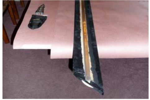
Next, work the ends. My best suggestion is to wrap and tack the material over the end and then make cuts with the razor to eliminate the excess so you don't have large bulges at the ends.
