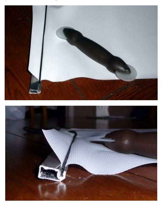
These 2 shots are to give you an idea of how the material and spline should seat into the aluminum rails.
