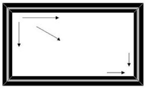
Once you've made it all the way to the far corner and the material is seated, look to see if you have any bulges or ripples. If you do, pull some of the spline and re-work the material to remove the imperfections. You may need to do this several times in order to take out all the ripples, but once done you will have a perfectly tensioned screen across the entire surface. And if it ever sags you can easily re-tension it.
