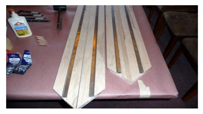
Next, tape over the metal tracks and trim the tape to the width of the rails with a razor knife, then flip the boards over so the viewing side is facing up.
