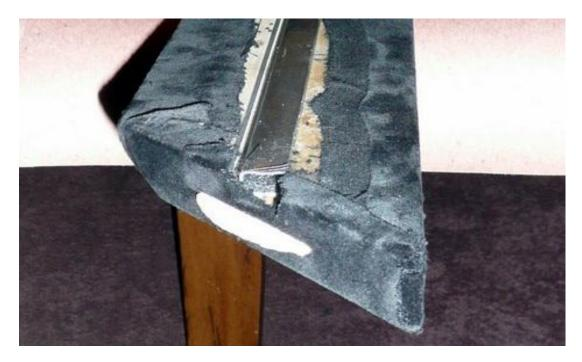
Carefully spray adhesive and tack down the end excess to the back. If you biscuit jointed the edges, carefully slice open the slot and insert the biscuit. You won't need to glue the biscuit in as the velvet will hold it in place nicely. Repeat this process with the other 3 frame sections.
