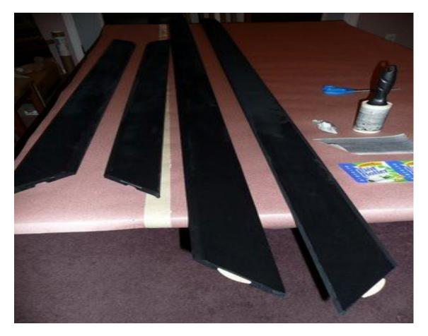
Once you've finished wrapping the velvet and given the adhesive 20 or 30 minutes to set up, use a lint roller to remove fuzzies.
