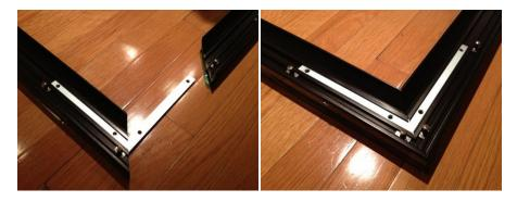
**Install last short side.** For this last piece, a short side, insert its L-brackets but do not tighten at this time. Align the four L-brackets into their mating slots into the top and bottom frame pieces and slide into position.
