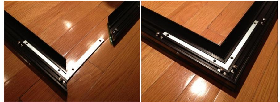
**Install last short side.** For this last piece, a short side, insert its L-brackets but do not tighten at this time. Align the four L-brackets into their mating slots into the top and bottom frame pieces and slide into position.
