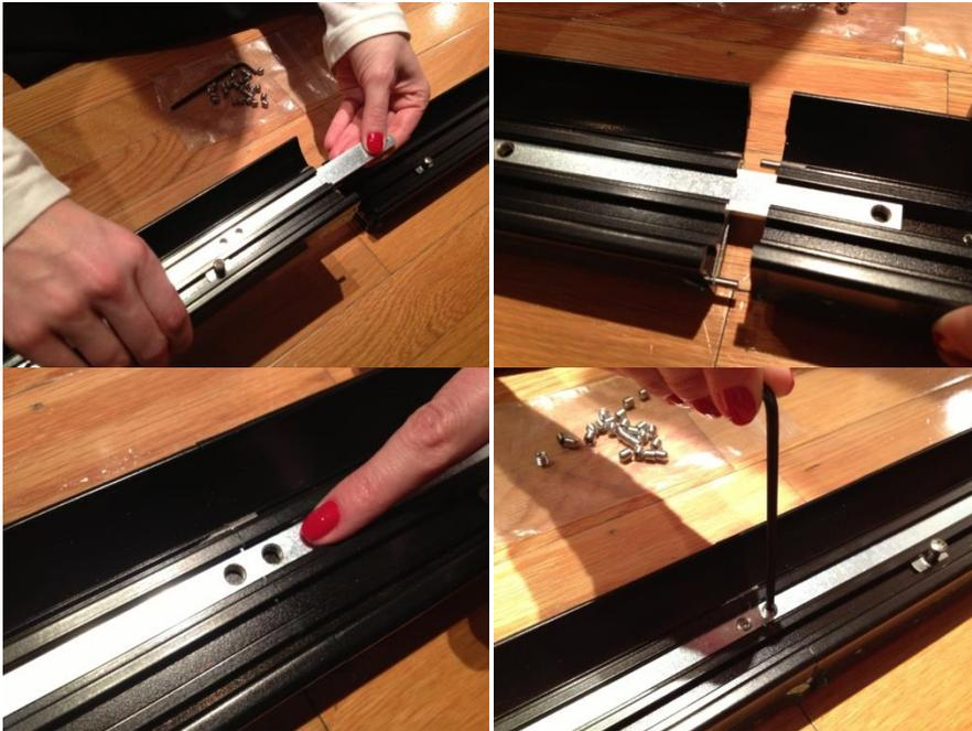
**Install L-brackets.** Align the L-brackets into their mating slots in the other frame member, and slide them together making a nice tight corner.
