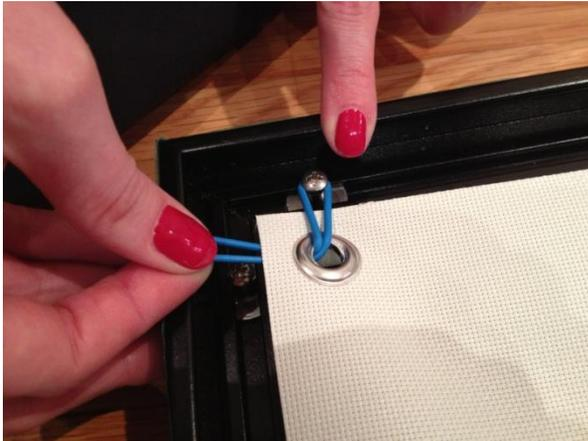
**Corner O-rings.** The corner o-rings will form an "L" shape across the corner grommets. Use 1 per corner.
