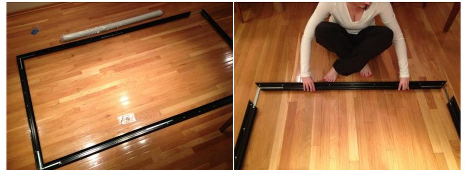
**Check alignment, then tighten screws.** Confirming with your fingers that the joints are aligned nicely, go ahead and tighten the remaining set screws.
